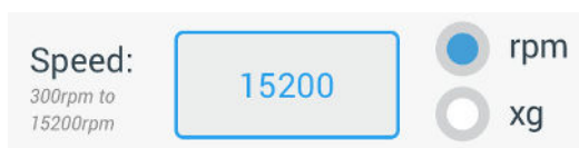
Figure 3-15: Setpoints Screen Detail for Centrifuge Speed, and Range
