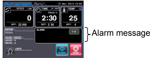
Fig.4-1 Displaying an alarm message
