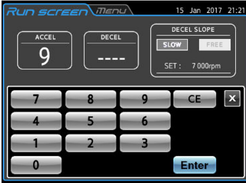
Fig. 2-2-4 (2) Setting screen (when DECEL SLOPE is set)
