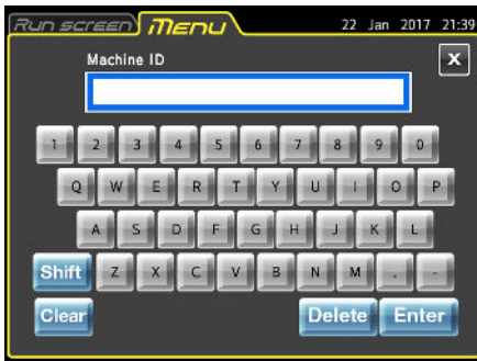
Fig. 2-5-4 (2) Machine ID entry screen
