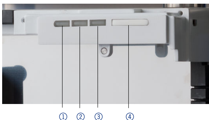
Fig. 18 LEDs and switch/standby button on the front of the device
