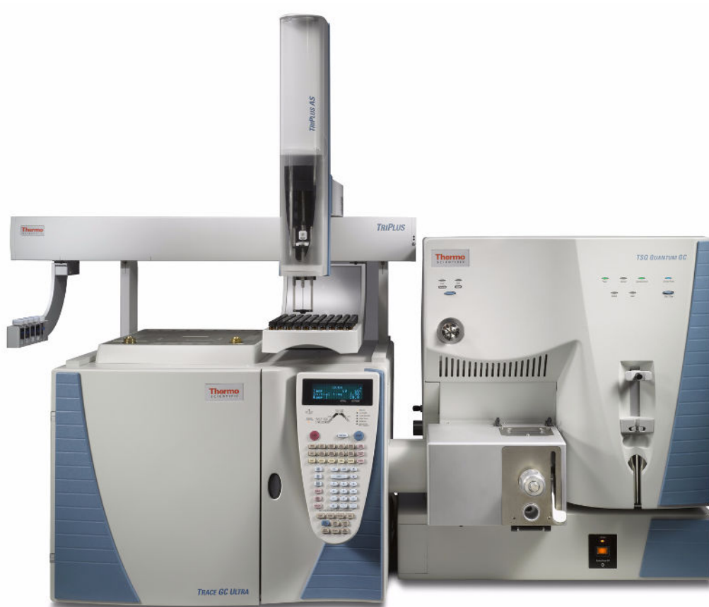
Figure 1. TSQ Quantum GC mass spectrometer, TriPlus autosampler, and TRACE GC Ultra gas chromatograph
