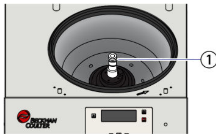
Figure 4.1 Lubricate the drive shaft
